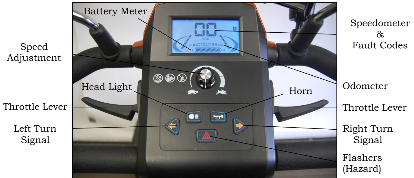
Figure 5. Delta Tiller Control Panel with LCD Display
