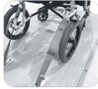
Fitting the rear restraint
