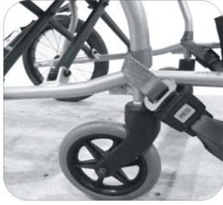
Fitting the front restraint
