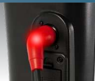
Magnetic charging with CHARGE360 technology
